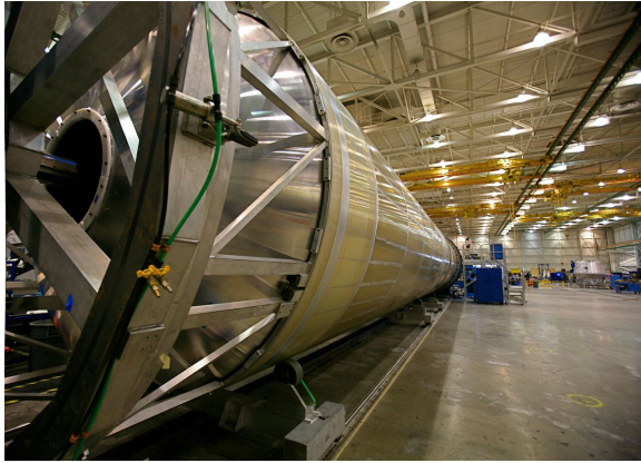
(a) Falcon 9 booster tank made of aluminum lithium alloy with FSW joints [a]
