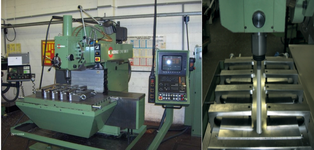
(a) Milling machine, modified for friction stir welding [a]
