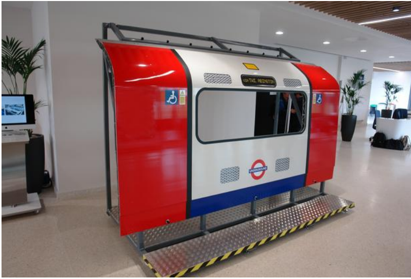
(c) FSW train panel of Bombardier's trains for London Underground [c]
