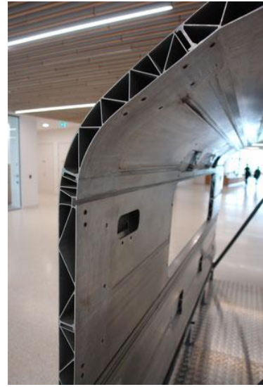
(d) Extruded aluminum panels joined with FSW [d]
