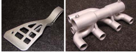
Figure 6: Typical parts produced by SLM circa 2009.
