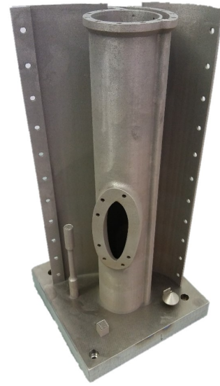
Figure 4.6: As-built SBA on a 160 \times 160 \times 30 \text{ mm} baseplate.
