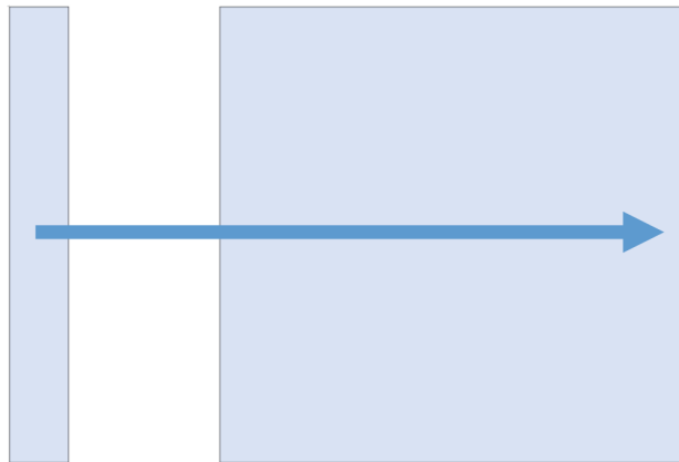
(b) Layer-by-layer: A new layer for the thin and the thick sample samples is simultaneously deposited in a single time step.
