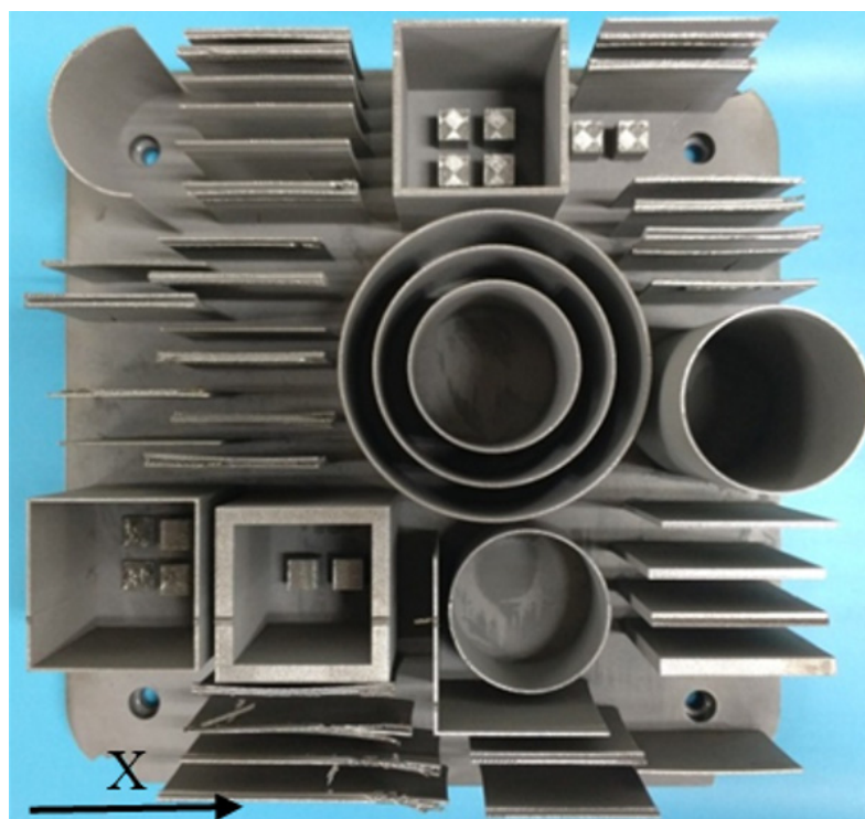
Figure 1. Typical thin-walled structures printed by LPBF.
