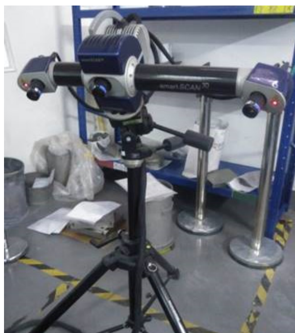
Figure 2. Breuckmann SmartSCAN3D scanner for the warpage measurements.
